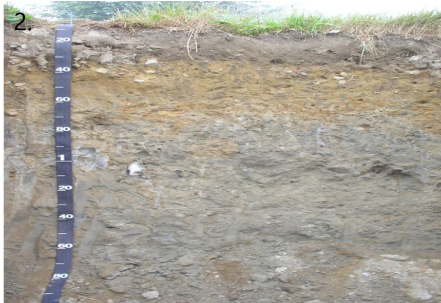
Photos of Maine soils. The first (1.) one shows an outwash soils with a finer textured topsoil layer. The second (2.) one shows a field profile typical in Maine where there is no organic horizon, just a plow layer. The third (3.) shows a spodosol, our most famous soil profile. We used to have a lot of these, but many have been destroyed by farming, forestry (skidding) or development. Note that all three show little rooting below the upper most layer of soil.
