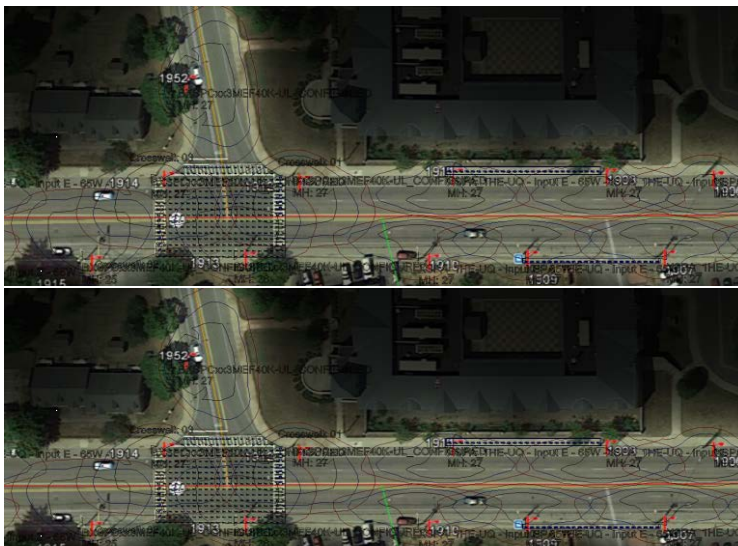
Figure 1: The sample graphic above is a digital rendering of RealTerm Energy's photometric calculations, taking into account the GIS inventory survey data and the lighting recommendations for the given street, intersection, sidewalks and pedestrian crosswalks.
