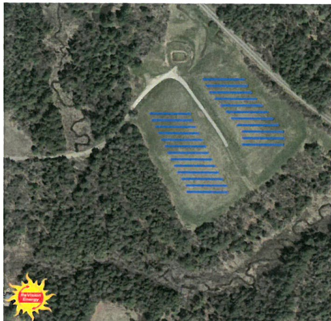
Preliminary 964.8 kW solar layout for the City's Ash Landfill
