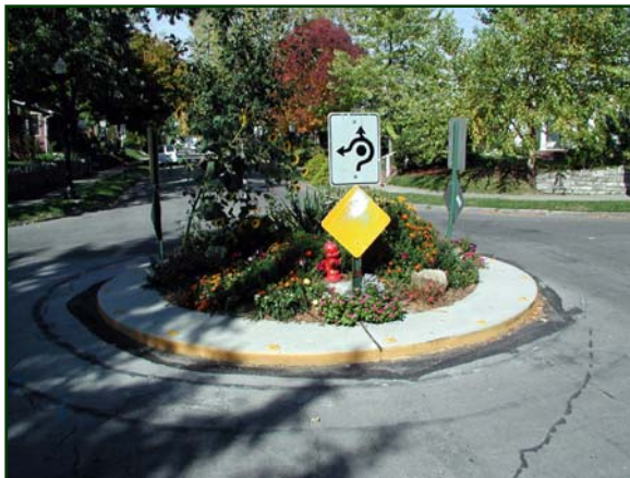
Figure 4.5: Neighborhood Traffic Circle/Mini-Roundabout
